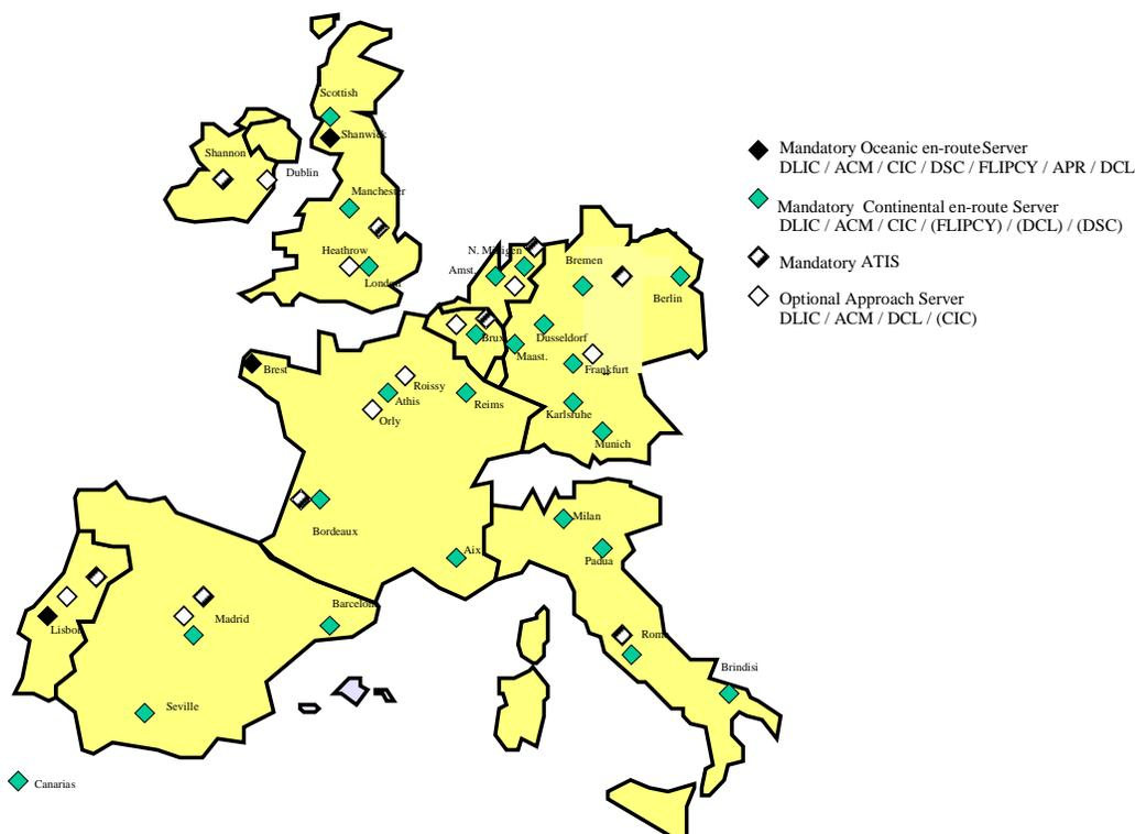
**Figure 3-2: Location of ATN Datalink Servers in the Initial ACCESS ATN**
