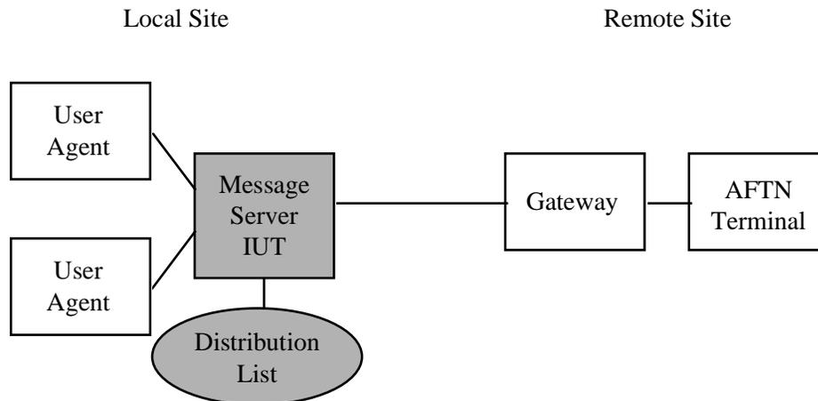
**Figure 5-5: Configuration 3 - message server to gateway**
