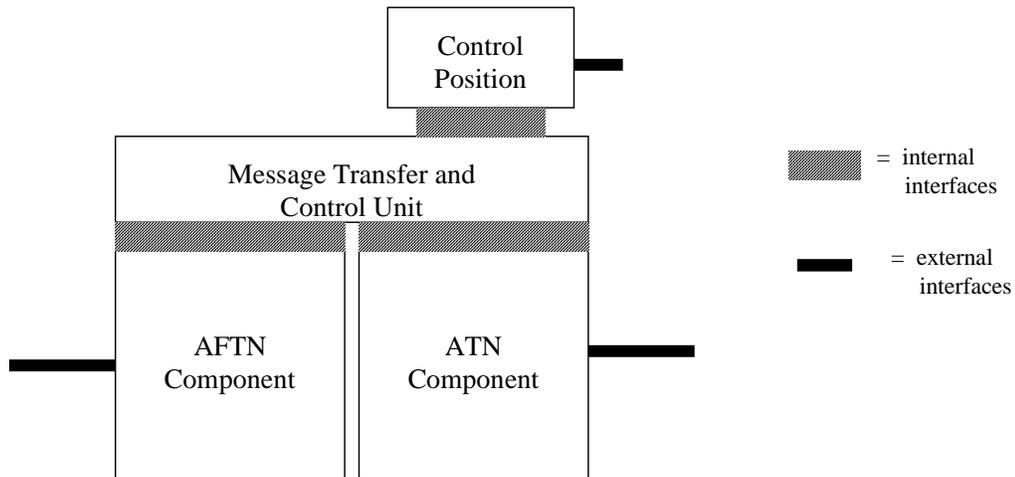
**Figure 5-8: Logical structuring of the Gateway**
