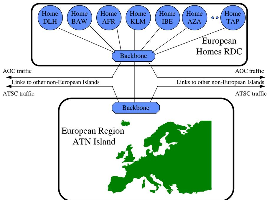
**Figure 2-1: Proposed overall Routing Architecture for the European ATN**
