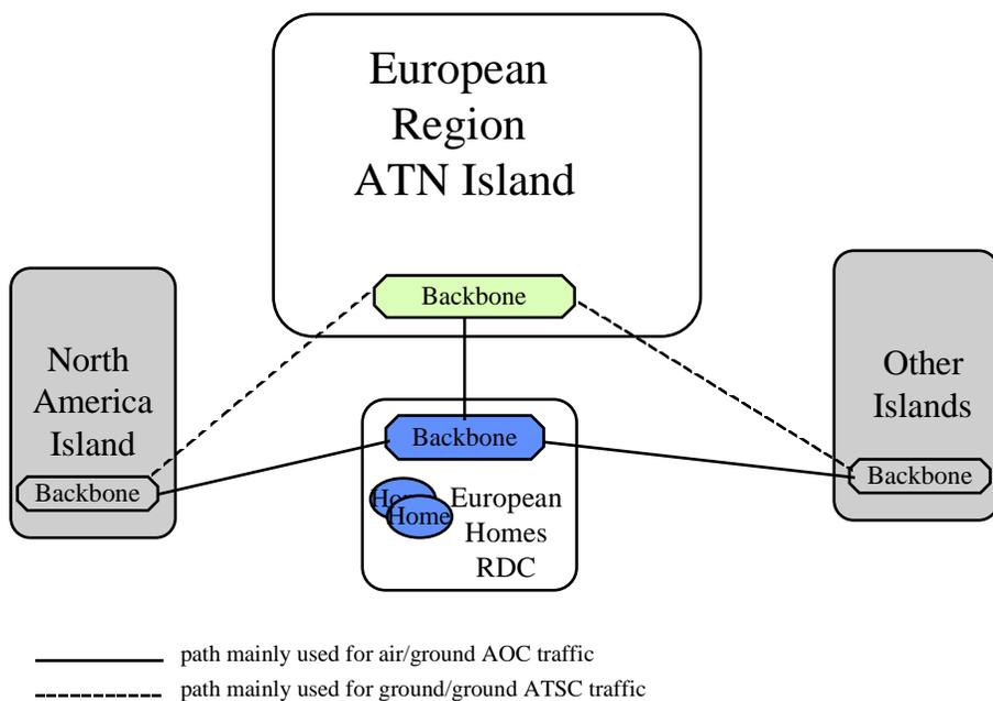
**Figure 3-3: Proposed Overall Architecture of the Initial ACCESS ATN**
