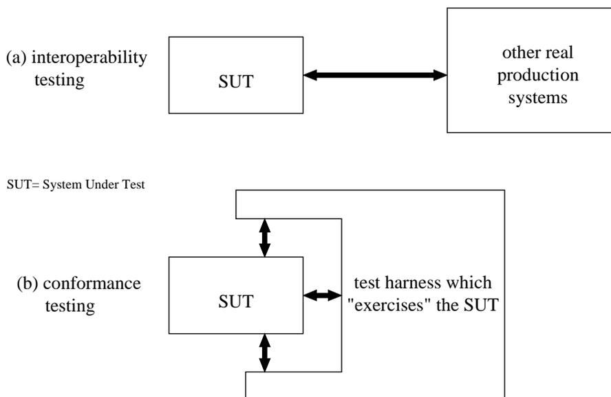
**Figure 5-1: Schematic distinction between interoperability and conformance testing**
