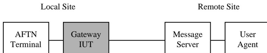
**Figure 5-4: Configuration 2 - gateway to message server**
