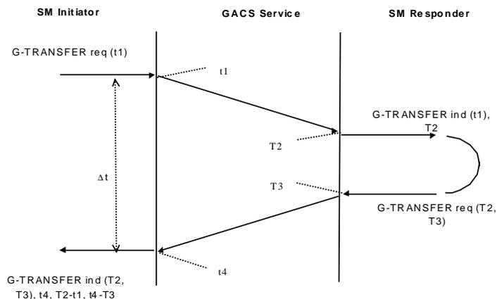
Figure 2. Automatic response supporting data integrity check and transit delay monitoring
