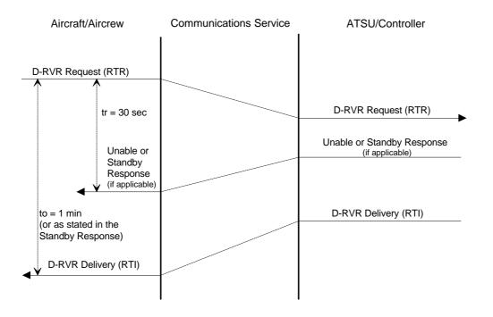
For the broadcast D-RVR service, the maximum time allowed from the composition of the RTR to the notification of the RTI to the Aircrew shall be [to = 1 minute].
