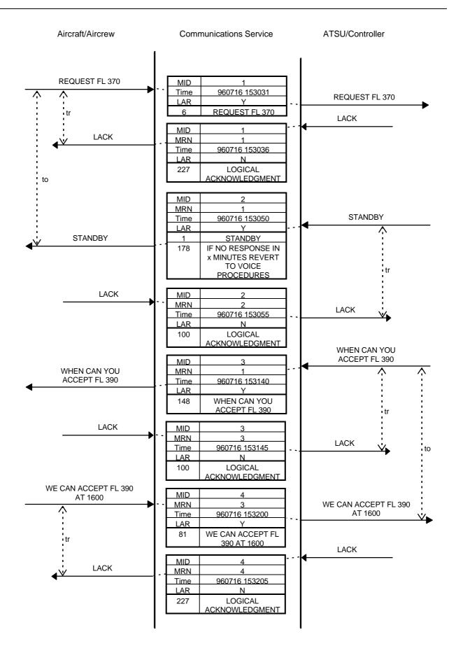
The previous data link exchanges end with the LACK to the "WE CAN ACCEPT FL 390 AT 1600" message because this message does not require a response (as required by the message RESP attribute specified in the message element description tables in subsection 8).
