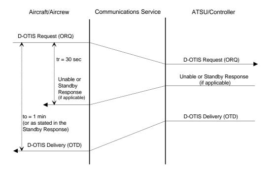
For the broadcast D-OTIS service, the maximum time allowed from the composition of the ORQ to the notification of the OTD to the Aircrew shall be [to = 1 minute].
