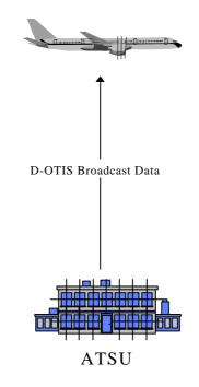
NOTE: The broadcast operating method is not supported in the "ICAO Manual of Air Traffic Services (ATS) Data Link Applications".
