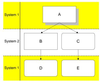
This diagram describes an exchange that can only be initiated on the generation of message "A" by System 1.
